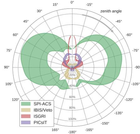
**Fig. 1.** Relative sensitivity of the different detectors on board INTEGRAL as a function of the photon arrival direction (Savchenko et al. 2017c). The shaded regions indicate the variation in sensitivity in the different azimuthal directions. A burst with duration of 1 s and Comptonized spectrum with  $\alpha = -0.5$  and  $E_p = 600 \text{ keV}$  has been assumed.
