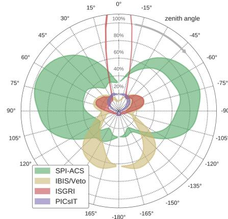
**Fig. 2.** Same as Fig. 1 but for a burst with duration of 8 s and a Band spectrum with  $\alpha = -1$ ,  $\beta = -2.4$  and  $E_p = 300 \text{ keV}$ . Note that in this case the IBIS/VETO provides a better sensitivity than the SPI/ACS for events coming from the bottom direction.
